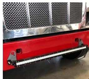
7. Finally wire up the supplied relay harness in the kit for the light bar. The output of the harness in Plug-n-play to the light bar connector. Wire 12+ volt power and ground to the harness and mount the switch in the desired location. *You may need to extend the wires to the switch depending on your desired mounting location.*
