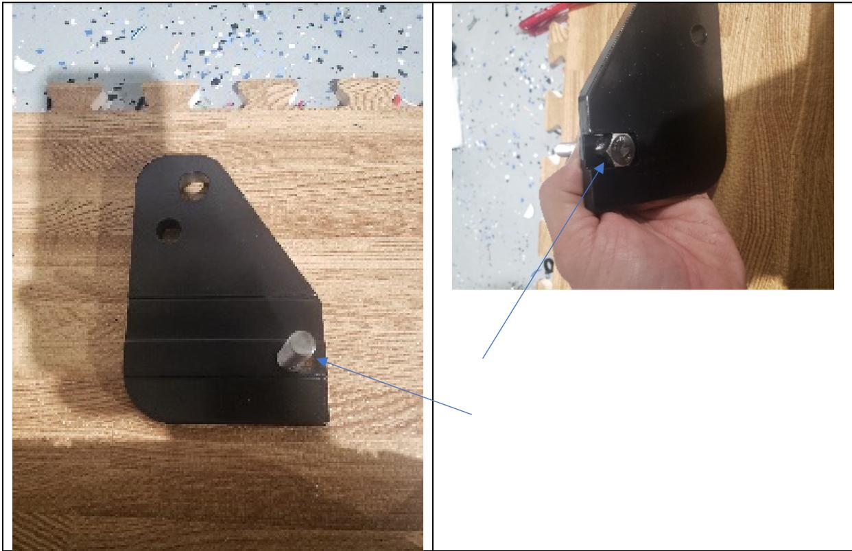
**4. Using factory bolts from truck, attach through bracket with bolt wedged between the bumper and bracket.**
