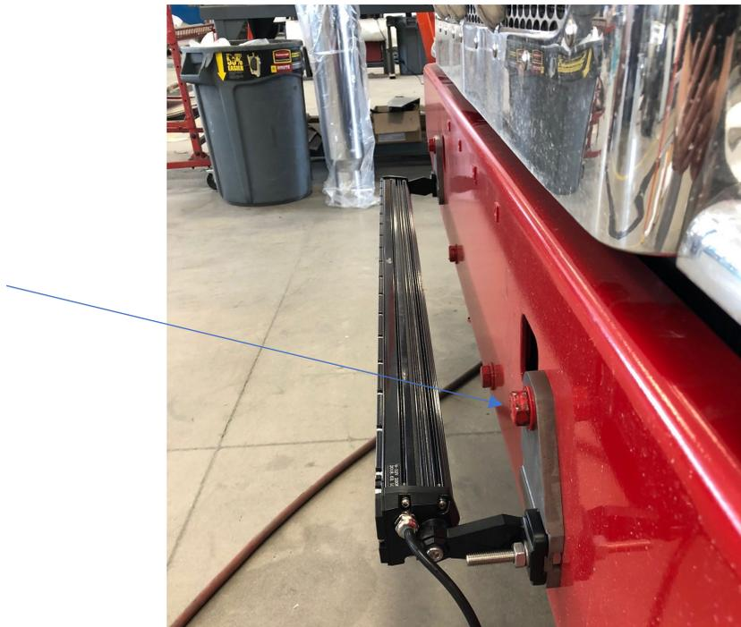
5. Assemble the light bar with Universal L-brackets with supplied hardware.
