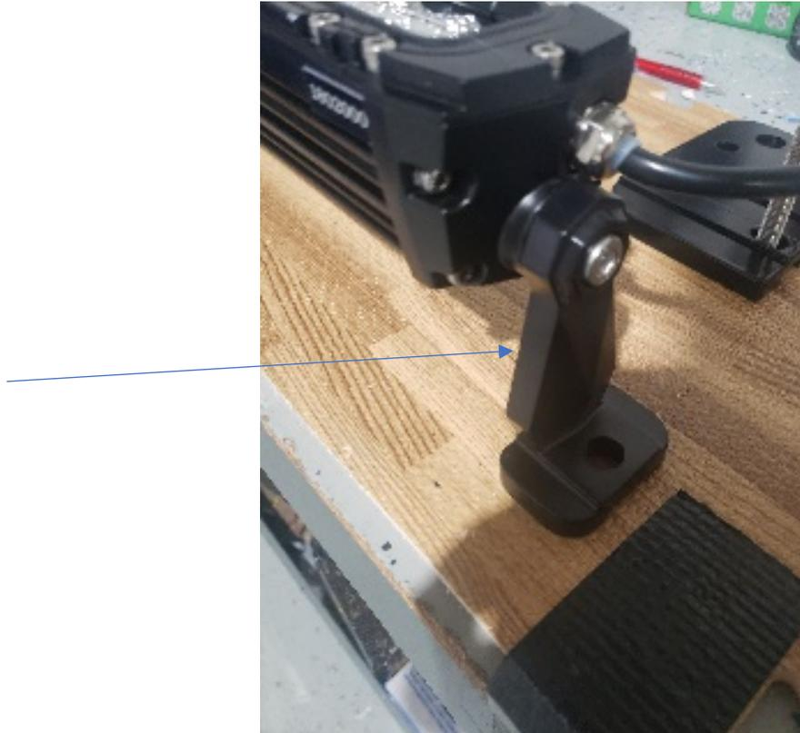
6. Align assembled light bar with bolts from bracket that is attached to bumper and assemble them with bolt washer supplied with kit. Once it is aligned secure and tighten all bolts and screws down.
