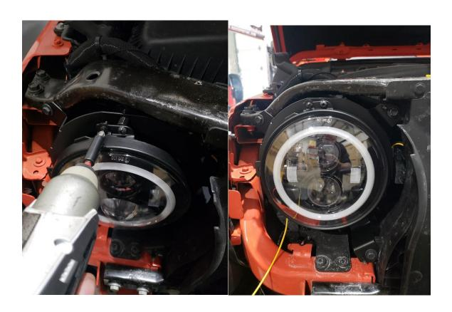
Test the new lights and make sure everything is functional, you may also check headlight adjustment if it off the you may adjust the headlights using the adjustment screw.
