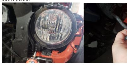
3. Once the assembly has been removed, you may plug in your adapters. One adapter is to convert the plug over to an H4 plug, the next plug is to interface the new 7" round to the vehicle.
