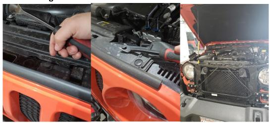
2. The next step is to remove the actual headlight assemblies by removing 10mm bolts (QTY.3), unplug factory plug from the headlight assembly and set it aside.
