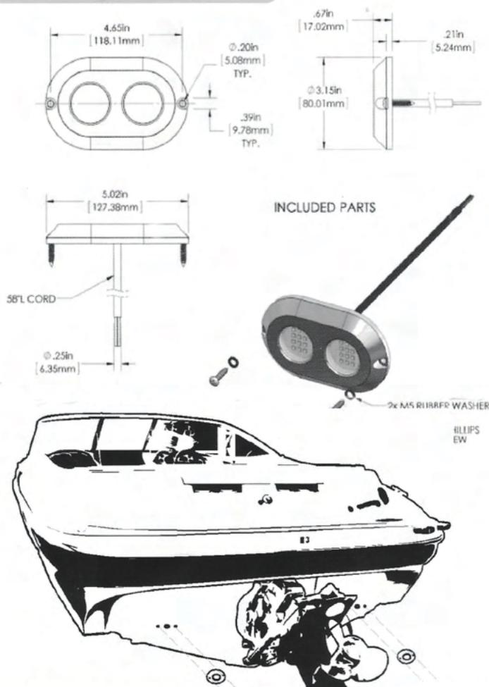
2. Drill 5/16" through hole in center of desired location and feed power wire through hole into boat. Hold light flush against transom, mark location for mounting screws, then remove light. Drill pilot holes for mounting screws to prevent cracking in fiberglass hulls.
