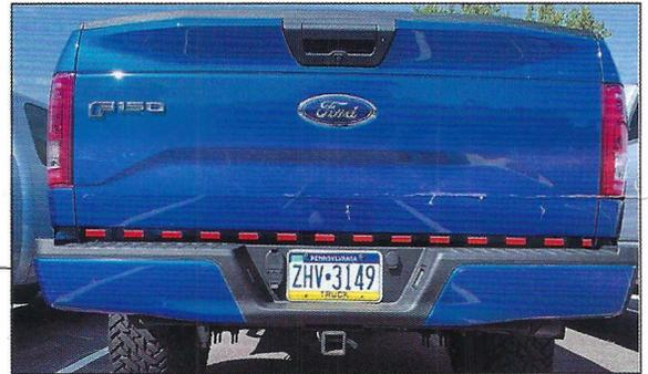
Next, locate a suitable mounting position for the light bar. Typical installation is between the tailgate and the bumper. Preparation for installation; thoroughly wash and dry the mounting location using an automotive grade soap and water. Ensure that you give the surface enough time to dry prior to installing the light bar. It is recommend that you wipe the mounting locations with isopropyl alcohol to ensure a wax and grease free mounting surface. \*\*Do not use silicone based cleaners.
